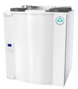
The unit is equipped with outputs to control an external hot water battery and inputs prepared for demand controlled ventilation from external sensors, e.g. CO2, presence or humidity sensor (potential free contact). Unit is delivered with built in moisture sensor that not only provides you demand controlled ventilation as standard but also is used for detecting and control defrosting in colder climate
