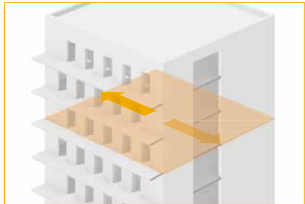
Movement direction parallel to insulating joint.
