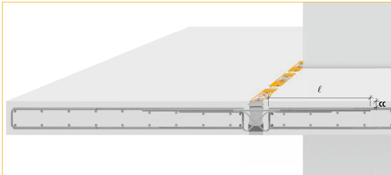
Schöck Isokorb® type CM: Overlap length l , concrete cover cc
