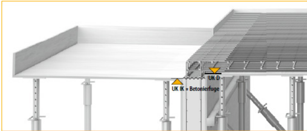
Figure 2: placing of Isokorb on formwork
