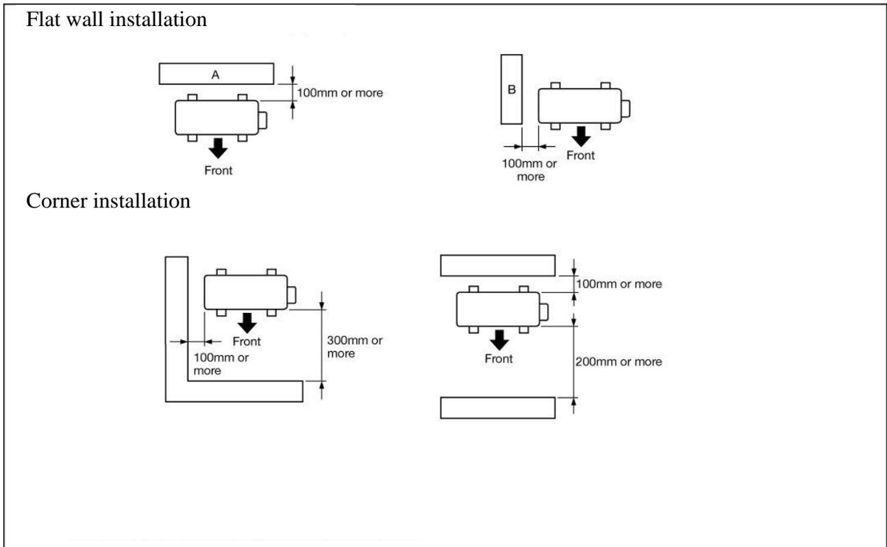
**Figure 4: Restrictions on installation with the space between the tank unit and the heat pump unit**
