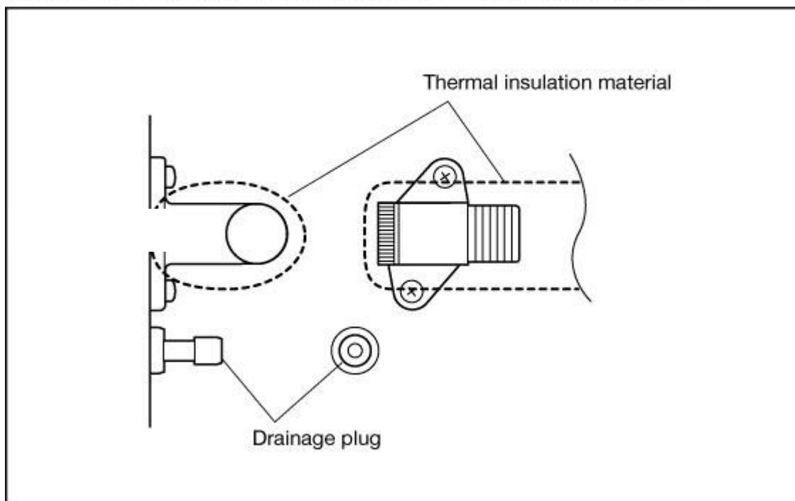
\* Do not wrap thermal insulation around the drain plug.
